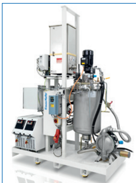
Fig. 3: The mixing and metering systems for PU systems that contain expandable graphite are equipped with a screw conveyor and a premixing station
