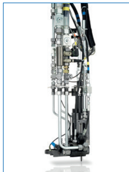
Fig. 4: In the MK8/12 ULKP-2KT-BP mixing head, the polyol component is fed to the mixing chamber through two opposing nozzles (T-mixing)
