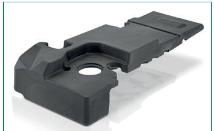
Fig. 2: Adding expandable graphite as a flame retardant improves also the noise-reducing property patterns of PU parts
