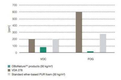
The typical average values of volatile organic compounds (VOC) and fogging content (FOG) measured for OBoNature™ products are clearly lower than those of comparable ether-based PUR foams and also below the limits of the VDA 278. (Graphic: FoamPartner)
